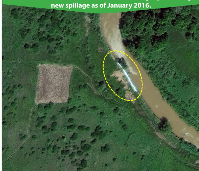
The bright linear feature indicated with yellow circle is the reinforcement of the embankment (sand bags) preventing a new spillage as of January 2016.
