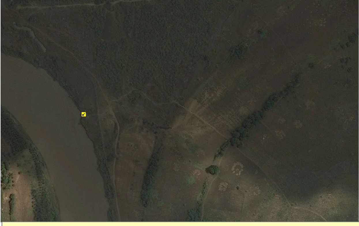
Sciongolo Dunia (30th Aug 14) - In 2012 a breakage was present, producing a major flooding. The image of 2013 is covered by clouds. In Jan 2014 the breakage is visible and seems to be opened. In May and Aug. 2014 signs of flooding are detected but the breakage seems to be closed.
