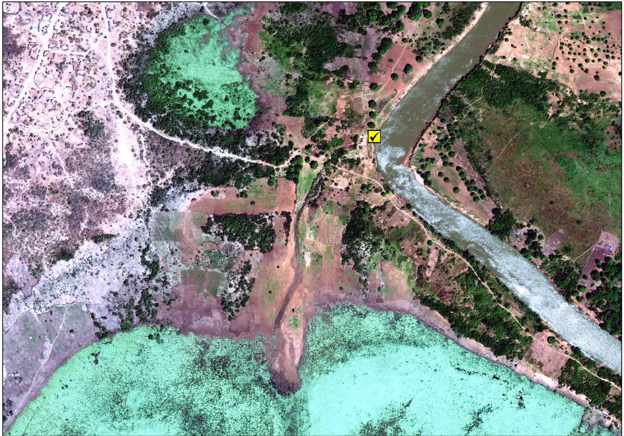
Raxoole (3 Feb 12) - In Feb 2012 signs of a flood are evident. Water spillage may have taken place from this point. The lack of embankments make this point vulnerable.
