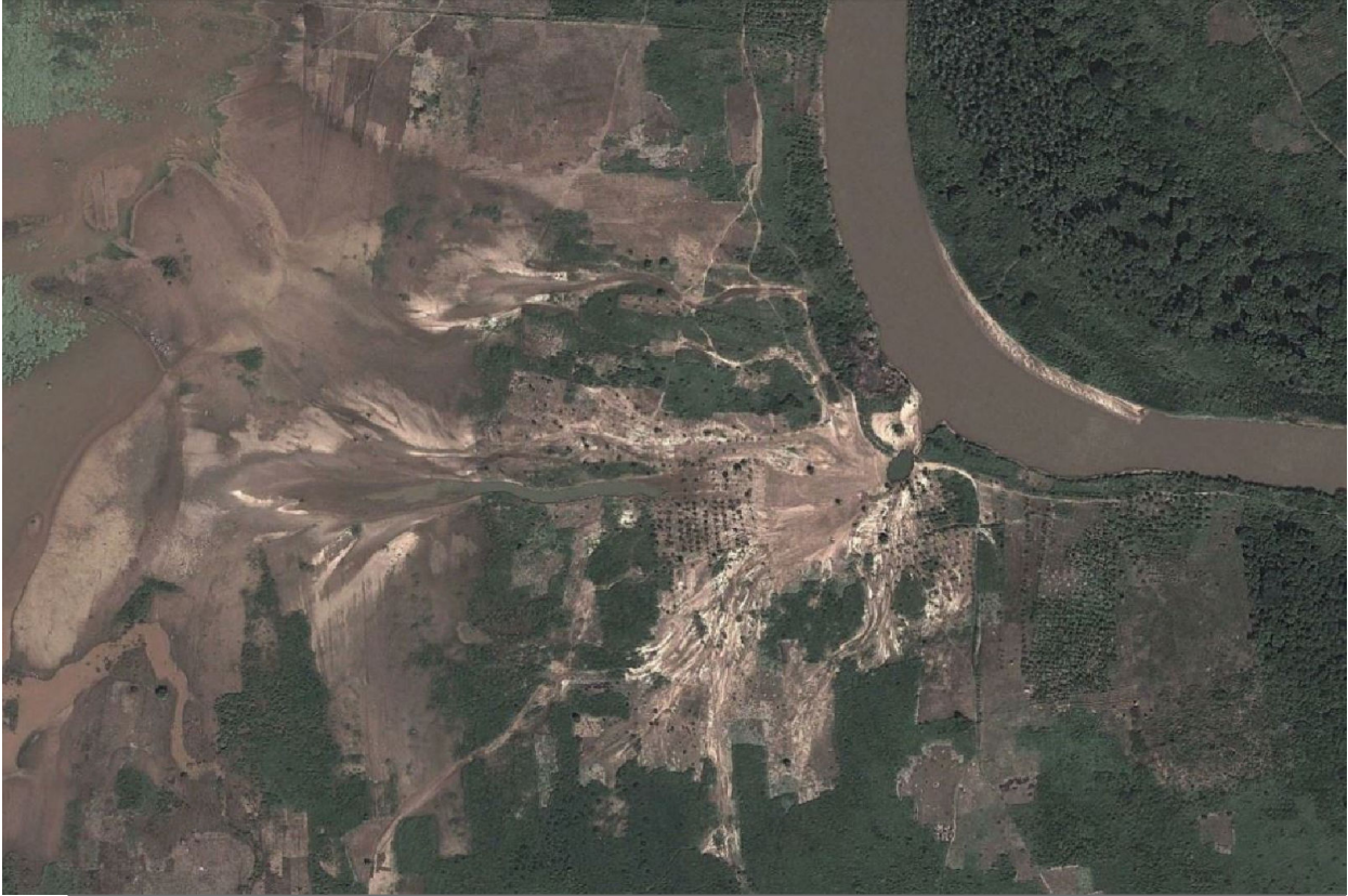
Cusmaan (1st Jan 14) - In 2012 and 2013 presence of sediments indicate that overflows occurred from this point. In late 2013 a major flooding occurred but no mitigation measures (embankments) are noticed as of March 2014. DEM and previous reports confirm this vulnerability.
