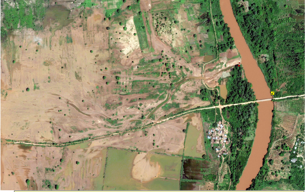
Muuna (18 Dec 13) - In Nov 2013 there is evidence of an active breakage at this point causing a major flooding. DEM and image of 2012 shows vulnerability. Images of 2014 show a minor fixing of the breakage, so it is still considered potentially vulnerable.
