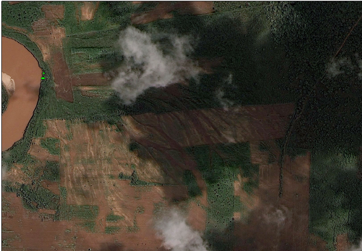
Seylac (24 May 14) - The image of Jan 2012 clearly shows that a breakage was present in this point. In late 2011 and a huge flooding took place. In 2013 and 2014 the breakage is closed. In May 2014 the area is flooded but the spillage is not coming from this point.
